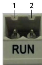
Fig. 20: Terminal pair RUN
