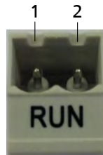
Fig. 22: Terminal pair RUN
