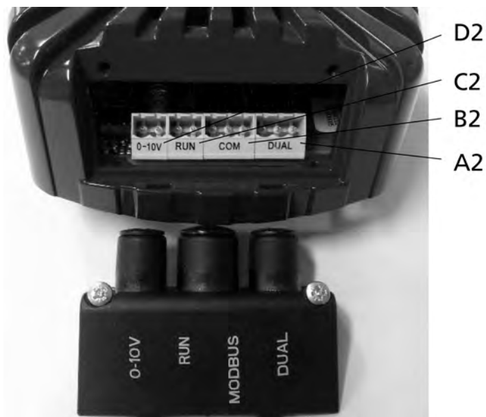
Fig. 5: Terminal wiring compartment for the data cables
