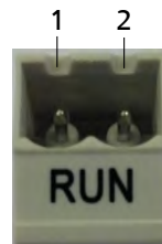
Fig. 26: Terminal pair RUN
